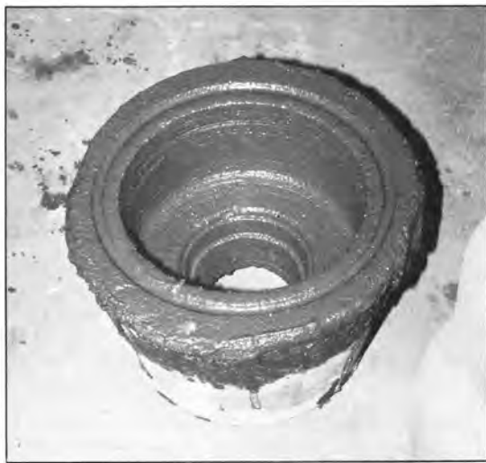
3. The completed outer mold before the final applications of fine, sieved mane .
