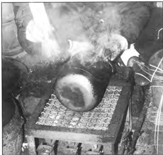
15. The kettle is heated and a lacquer glaze is applied.
