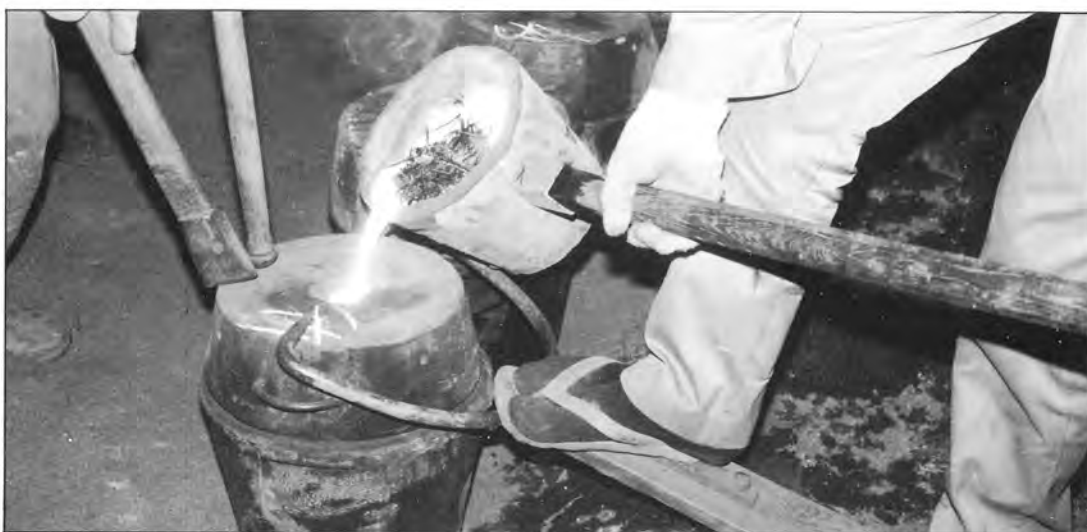
11. Molten iron is poured in through a hole in the center of the bottom half of the outer mold.
