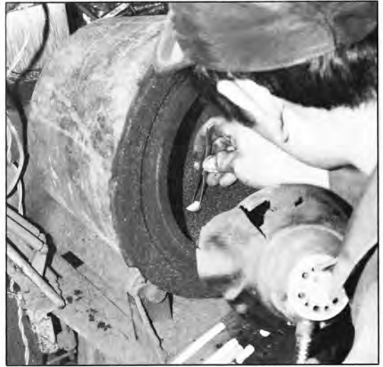
5. Lug dummies are buried in the wall of the outer mold.
