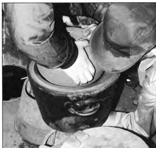
9. The inner mold is placed in the upper half of the outer mold.
