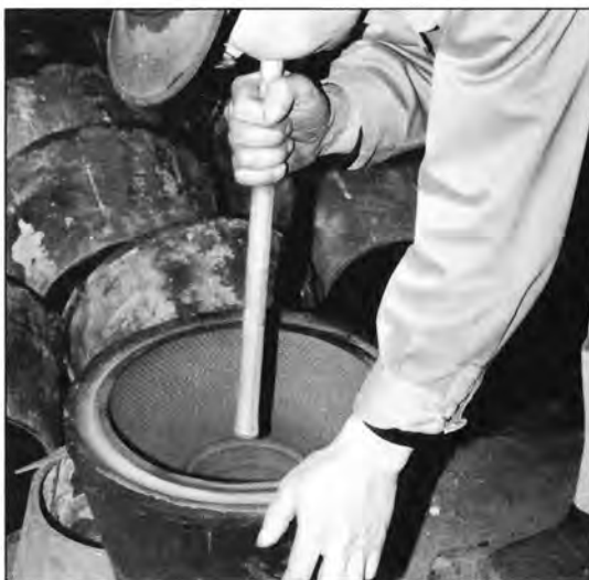
8. Using a length of bamboo, dust and any other debris is blown out of the mold to ready it for casting.
