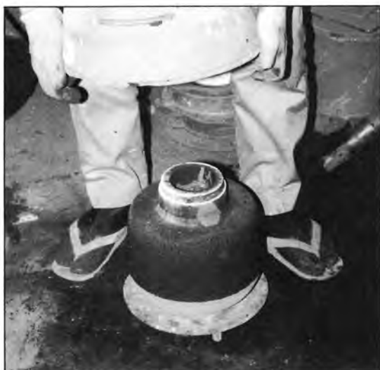
7. The inner mold is cast in the outer mold, fired, and then removed for shaving.
