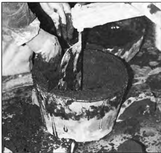
2. The kettle template is turned inside the outer mold to give it the proper contours.
