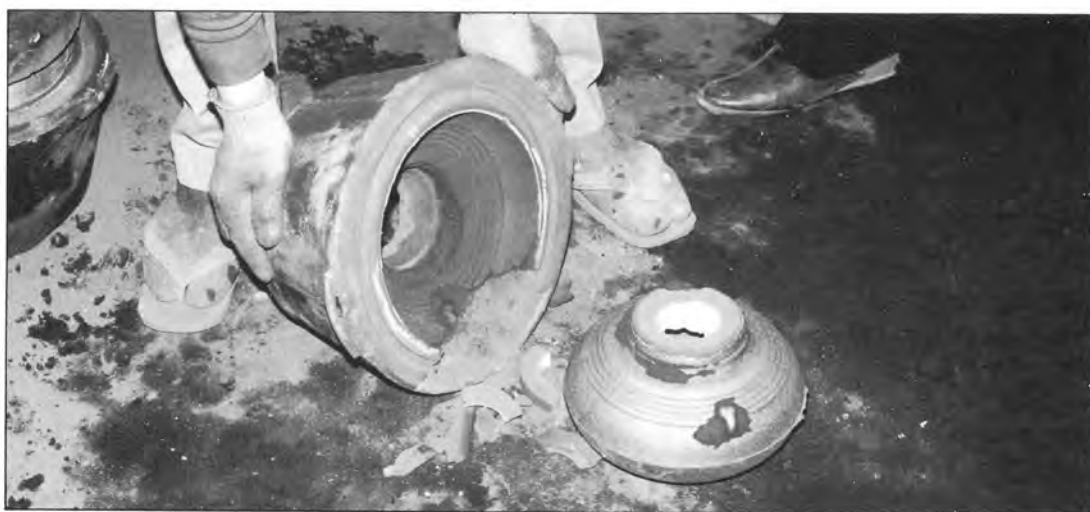
12. The kettle is removed from the outer mold. The inner mold still remains to be broken off the kettle body.
