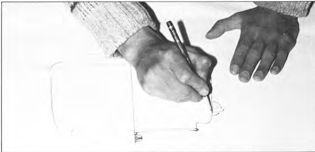
1. A drawing of the profile of the proposed kettle is made. Photos courtesy of Negoro Moshō and Rikogakusya Publishing Co., Ltd.
