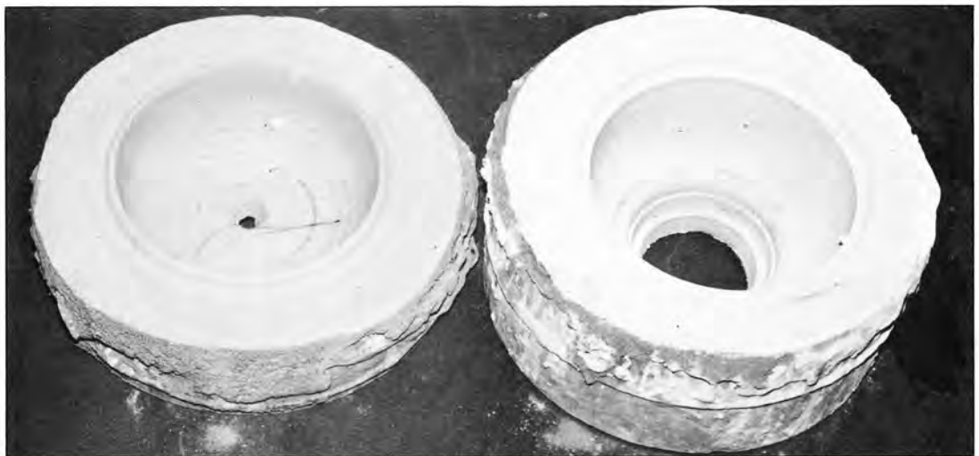
6. The completed outer molds are fired together and then allowed to cool.
