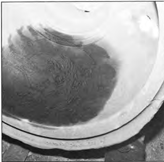
4. A design for the body of the kettle is worked into the inside surface of the outer mold.
