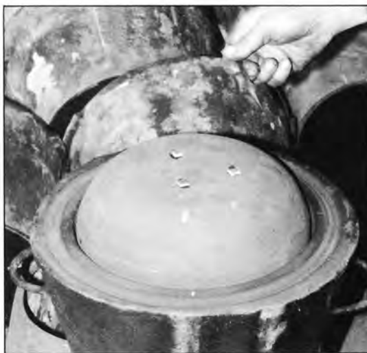
10. Small pieces of iron are placed on the inner mold to keep it from rising during the casting process.
