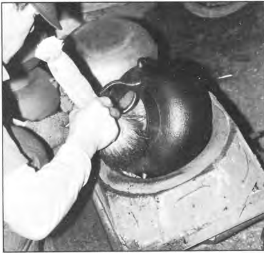
16. The lacquer finish is brushed with a wet brush to complete the body of the kettle.
