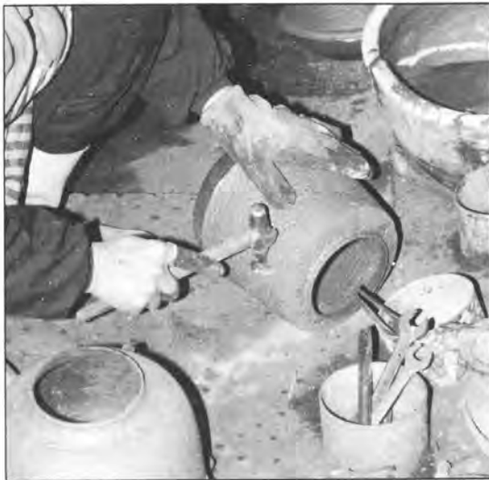
14. Small surface flaws that remain from the casting process are hammered off.
