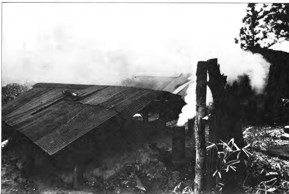
Above: Smoke rising from the chimney. An experienced sumi-maker can tell, from the smoke, how the burning process is coming along. Below: The kiln door, sealed with mud. When the wood has carbonized to the proper degree, the kiln is sealed air-tight, to smother the fire. The kiln is then allowed to cool to the point that there is no further chance of combustion.
